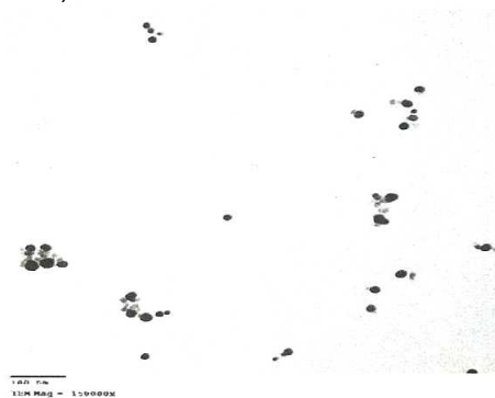
Fig. 3. TEM micrograph of the silver nanoparticles synthesized by A. ochraceus . Scale bar = 100 nm
